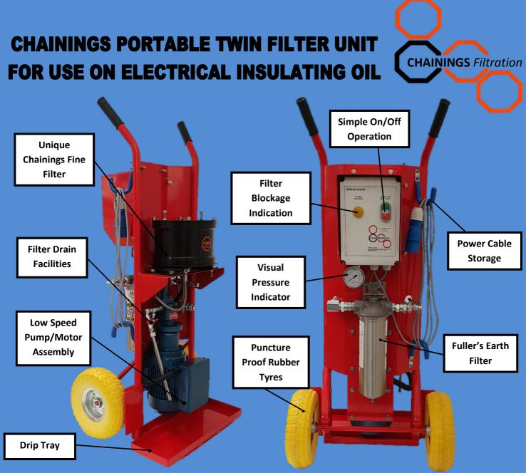
Designed for application on oil based Tapchanger and Transformer Systems.
